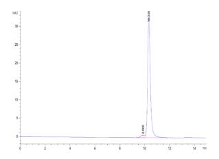
The purity of Mouse IL-1 Beta is greater than 95% as determined by SEC-HPLC.
